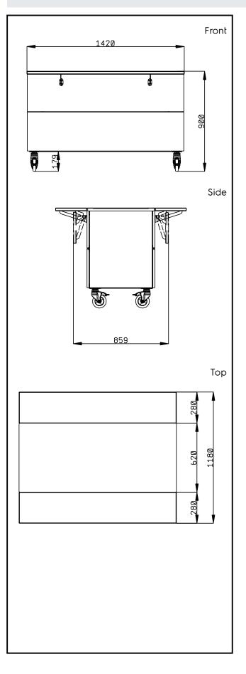
Flexy Compact Ambient unit on cupboard (4GN) with wheels, H=900mm
